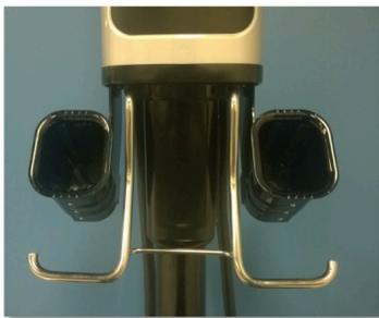
Attach the holster to the Head unit using the four (4) screws (2 for each side).
